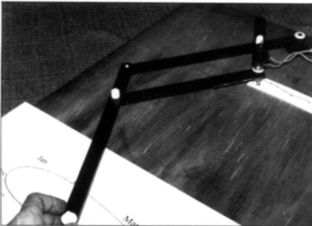
5. Engraving an analemma plate using a children's pantograph.
