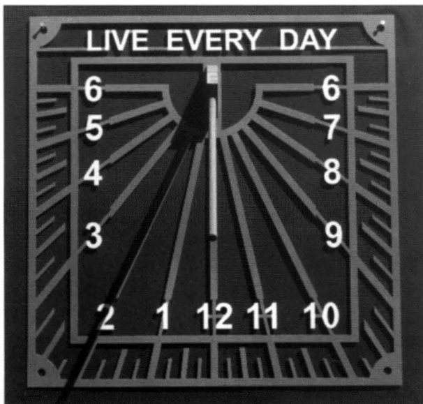
Figure 2. Laser cut, stainless steel wall sundial, 500x500x3 mm.
